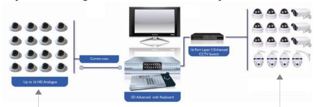
Up to 16 HD 720P Analogue Ice2 or standard definition analogue cameras connected directly to the unit
